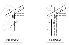
OVERHANG SOFFIT DETAILS 6.01 SCALE: 1/4" = 1'-0"
